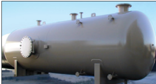
Properly sized hydropneumatic tanks are often bigger than most people may think. Tanks that are too small are dangerous, as they provide very little protection and a false sense of security.
