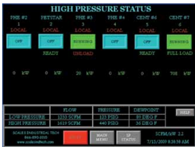
The $mart Sequencer® Main Menu button on the status screen provides real-time scfm/kW metrics to analyze the efficiency of the compressed air system
