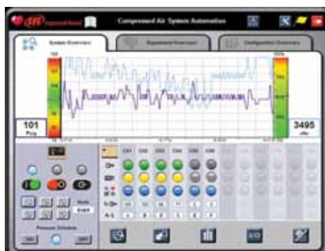
The Ingersoll Rand Xi-Series Visualization Module provides graphing of key performance data over time to help effectively monitor system performance
