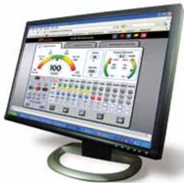
The Ingersoll Rand Xi-Series System Visualization Module provides operators with intuitive, graphic-based control of their compressed air system
