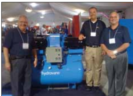
A Hydrovane Duplex package with two 10 hp rotary vane compressors mounted on a storage tank. Pictured are Bill Steele, Kurt Barhorst and Dean Chew (left to right)
