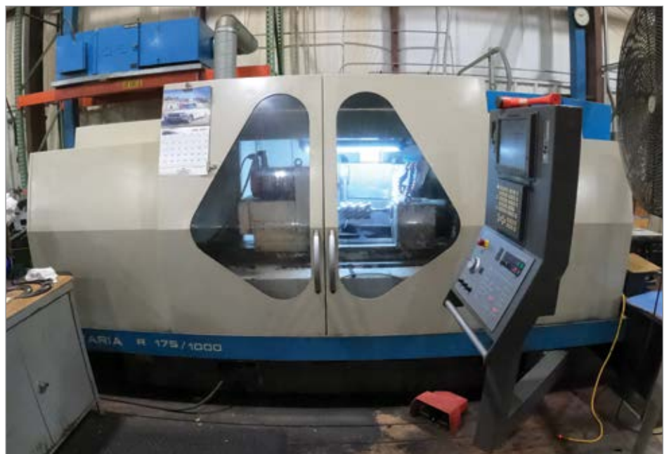
At its manufacturing plant in Michigan City, Indiana, Sullivan-Palatek uses high-precision CNC machines for milling and grinding blanks and converting them into male and female rotors for airends.
