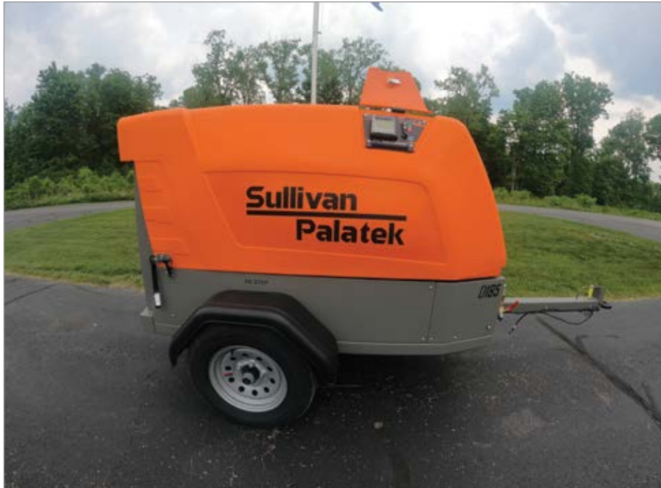
Sullivan-Palatek's upgraded portable air compressor line includes the D185PKR portable air compressor powered by 185 49-hp Kohler engine.
