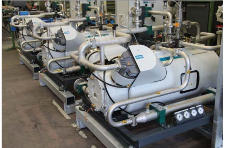
The hermetically gas-tight oxygen compressor HAUG.Sirius with water cooling can be operated reliably at high ambient temperatures. (© HAUG Sauer Compressors AG)
