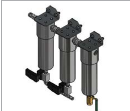
Filter assembly drawing for dual coalescing and carbon filters: maximum pressure 5000 psi (340 bar).
