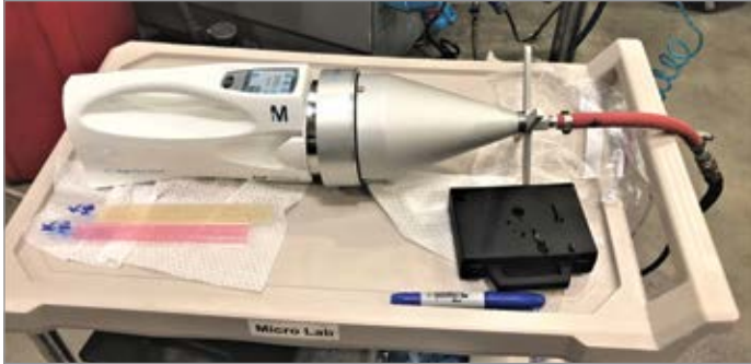
The Reuters Centrifugal Sampler [RCS] is a Slit type Impactor.
