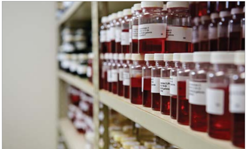
Testing each finished product and retaining a sample meets ISO 9001 procedures for ongoing validation of each batch.
