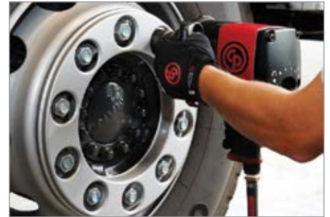
Pneumatic impact wrench installing tires.
