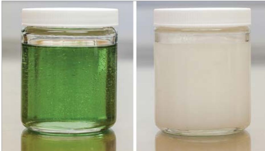
(LEFT) Example of two Compatible Fluids – once mixed, the fluid remains clear and bright with no residual film left above the fluid line. The green dye used in one of the fluids has had no significant impact on the fluids compatibility. The bubbles shown in the jar are what's known as air entrainment. These bubbles will rise to the surface and burst. (RIGHT) Example of Two Incompatible Fluids with Adverse Consequences – the common color and clarity impact can be seen in this example of incompatibility. The mixing of these two fluids have caused significant foaming to occur. Foaming can result in substantial fluid loss downstream, and cause the compressor's temperature to spike.
