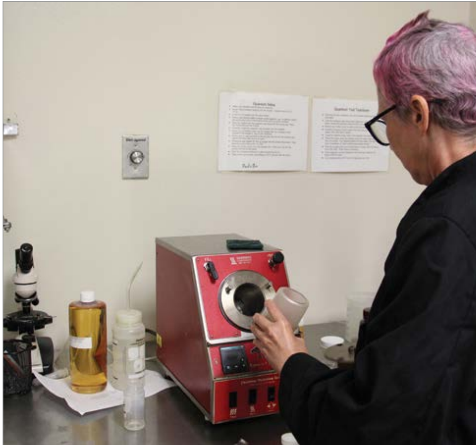
A senior laboratory technician at Isel Inc. prepares a sample for a RPVOT.
