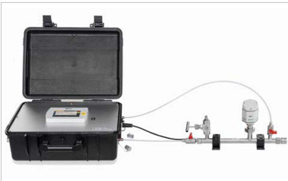
Shown is the SUTO iTEC's S600/AirCheck4 compressed air quality analyzer with an additional sampling unit for isokinetic sampling of particles. The isokinetic sampling device is used to sample air carried particles according to ISO 8573 (3) guidelines.
