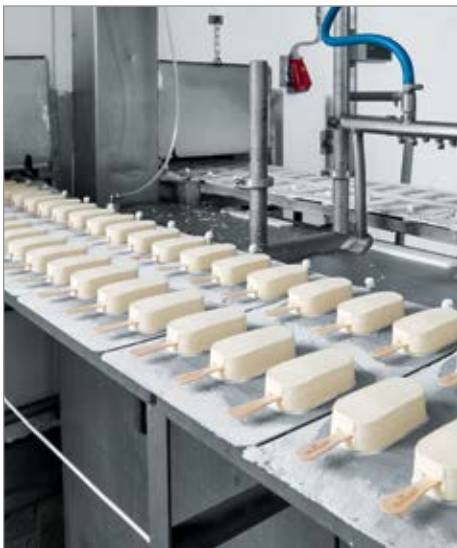
One production line at the Heppenheim plant produces more than 20,000 ice creams bars per hour.
