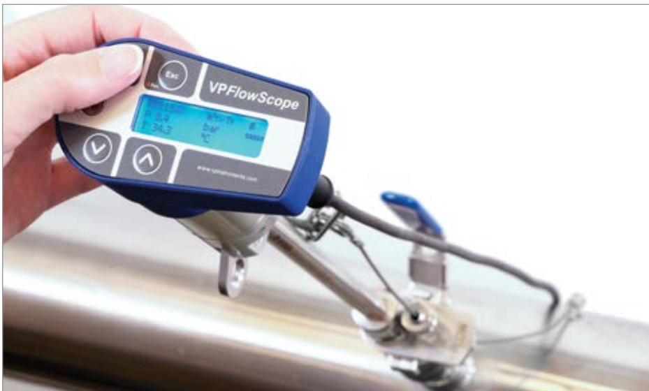
Flow meters installed on the glass manufacturer's compressed air system pointed to energy-savings opportunities.
