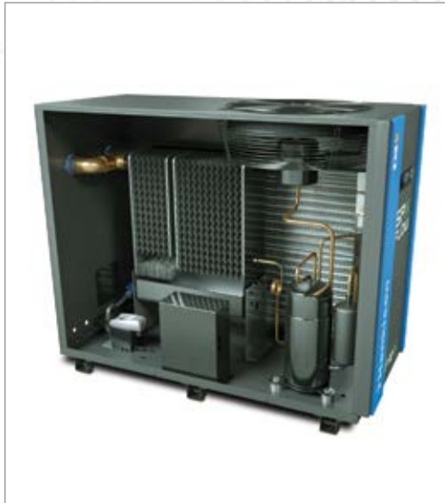
Refrigerated compressed air dryers use a refrigeration circuit and heat exchangers to condense and remove moisture from compressed air. Photo credit: SPX FLOW
