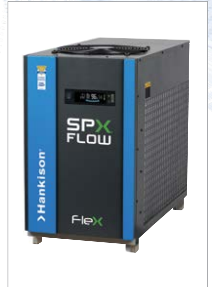
Refrigerated compressed air dryers use a refrigeration circuit and heat exchangers to condense and remove moisture from compressed air. Photo credit: SPX FLOW
