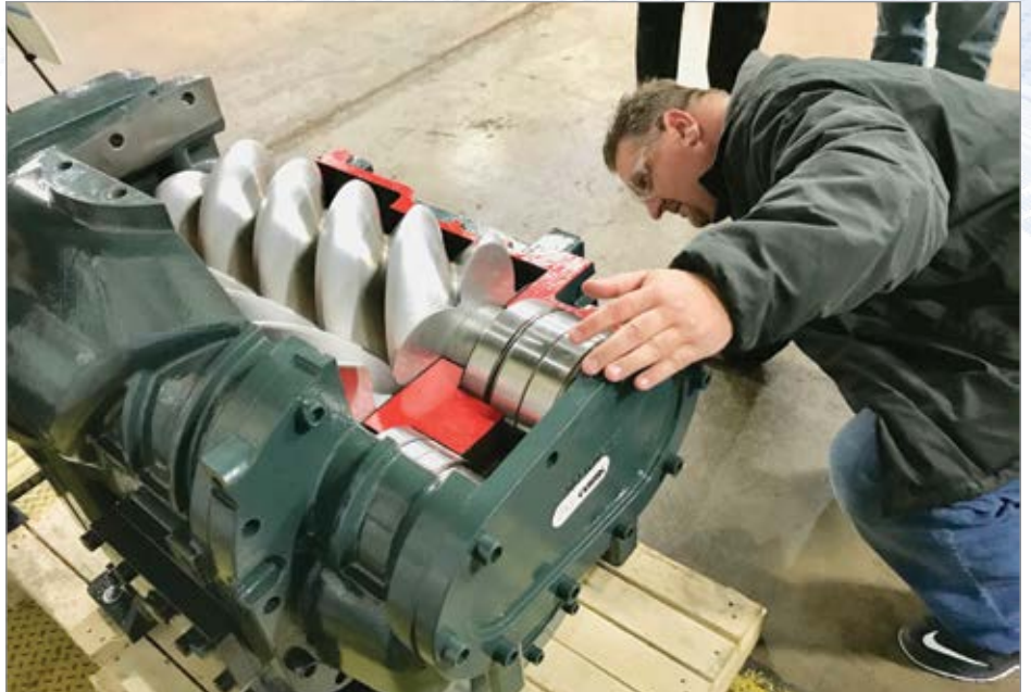
The job of an air compressor service technician requires a unique set of skills, such as understanding the heart of a rotary screw air compressor—the airend. Photo courtesy of Atlanta Compressor.
