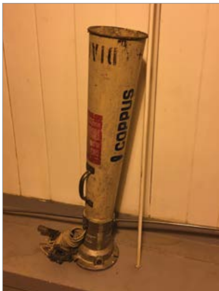
Figure 5: Devices like this compressed air-powered blowing horn were classed as possible inappropriate uses.
