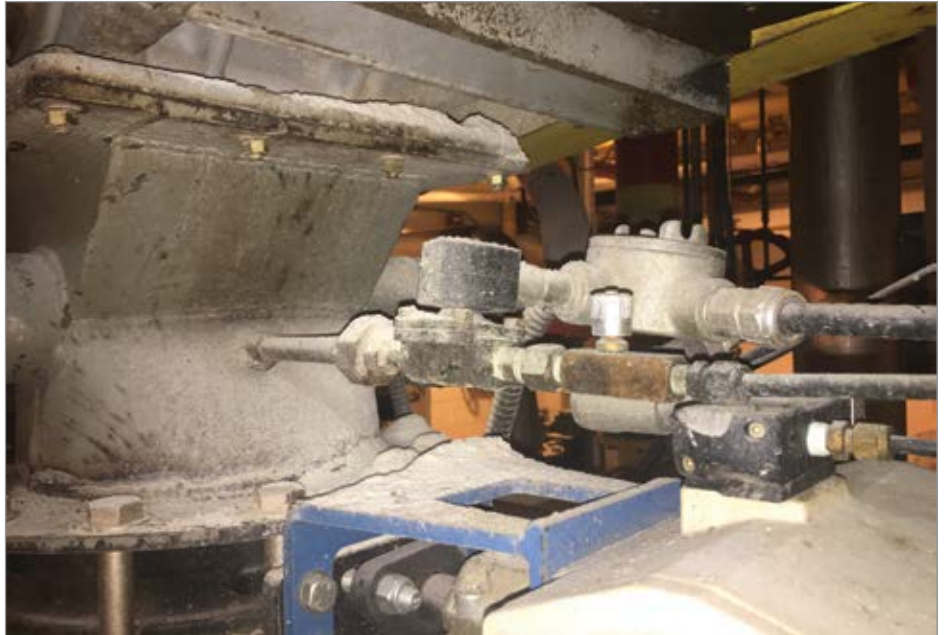
Star seals are used on the cooker as shown to meter the amount of ingredients going to the vessel.
