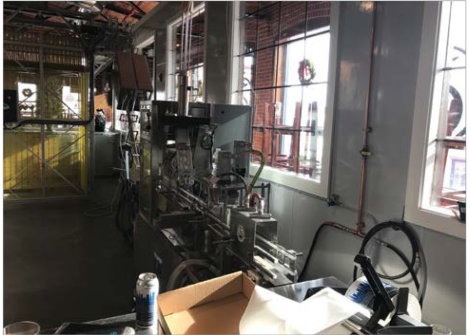
Five Churches' self-contained canning machine can fill, seam and lid up to 35 cans per minute.
