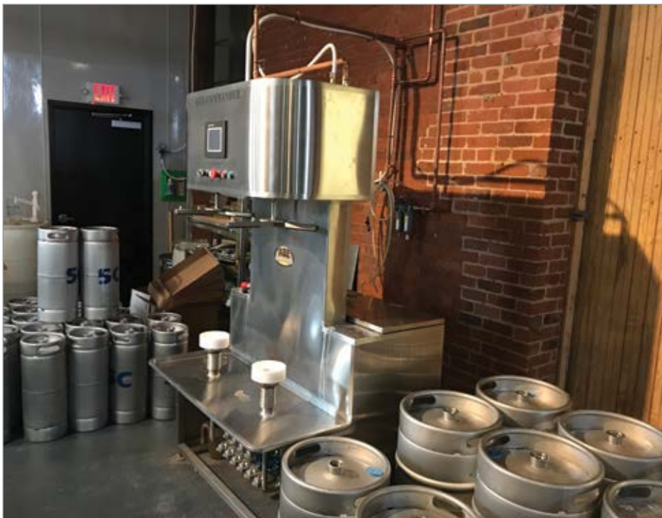
A keg washer eliminates the need for manual keg cleaning, while also ensuring availability of clean kegs.
