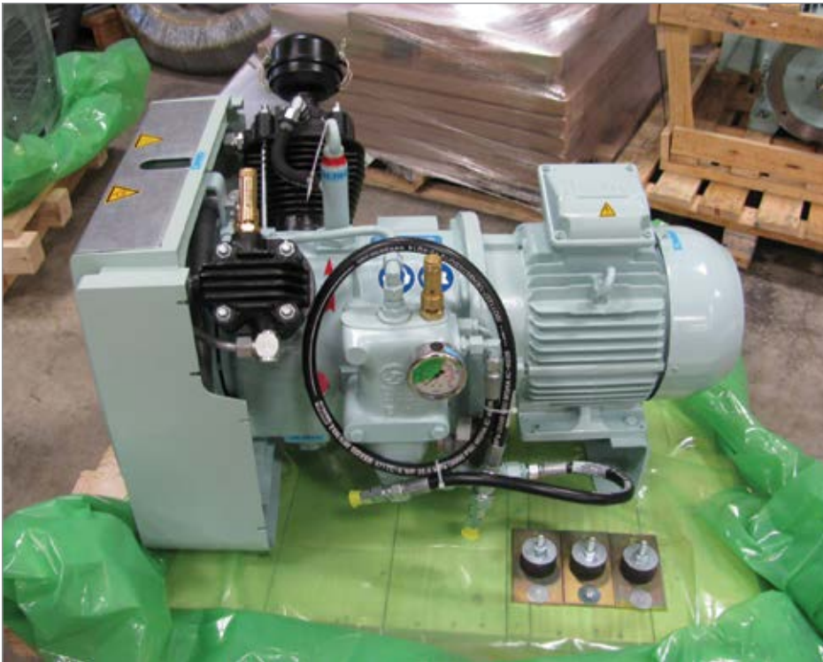
One of two WP22L compressors built for the USNS Bismarck at Sauer Compressors USA's factory just prior to shipping to Military Sealift Command.
