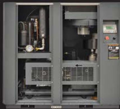
C-25 shown with integral dryer package.
