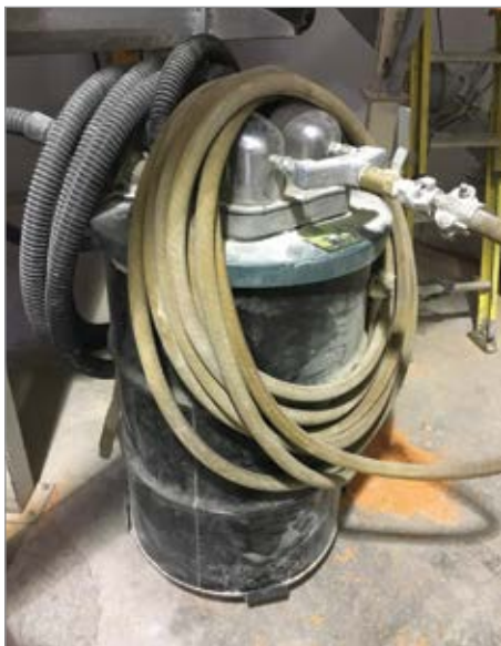
Figure 9: This compressed air powered drum vacuum adds to plant peak.
