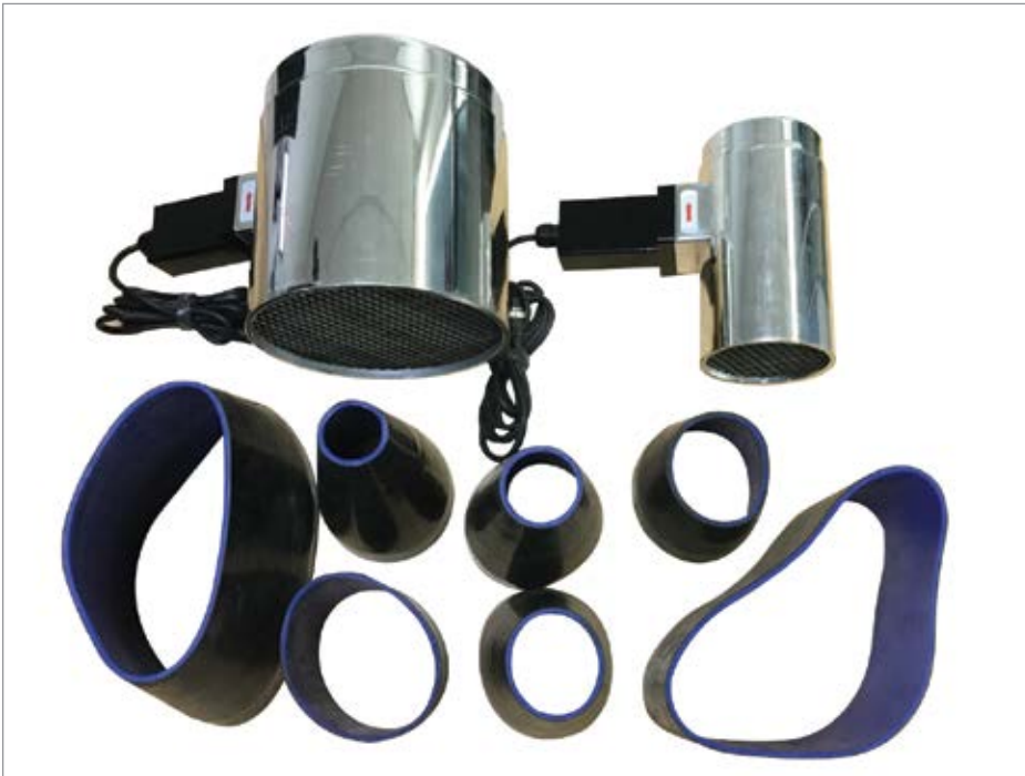
Typical intake flow meter with connection sleeves.
