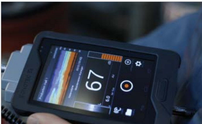
A typical leak on a compressed air filter unit is simple to analyze. The color-coded spectrogram, which shows the frequency (Y-axis) over the time (X-axis), shows a high amplitude (red color) in a range of 20 to 90 kHz.
