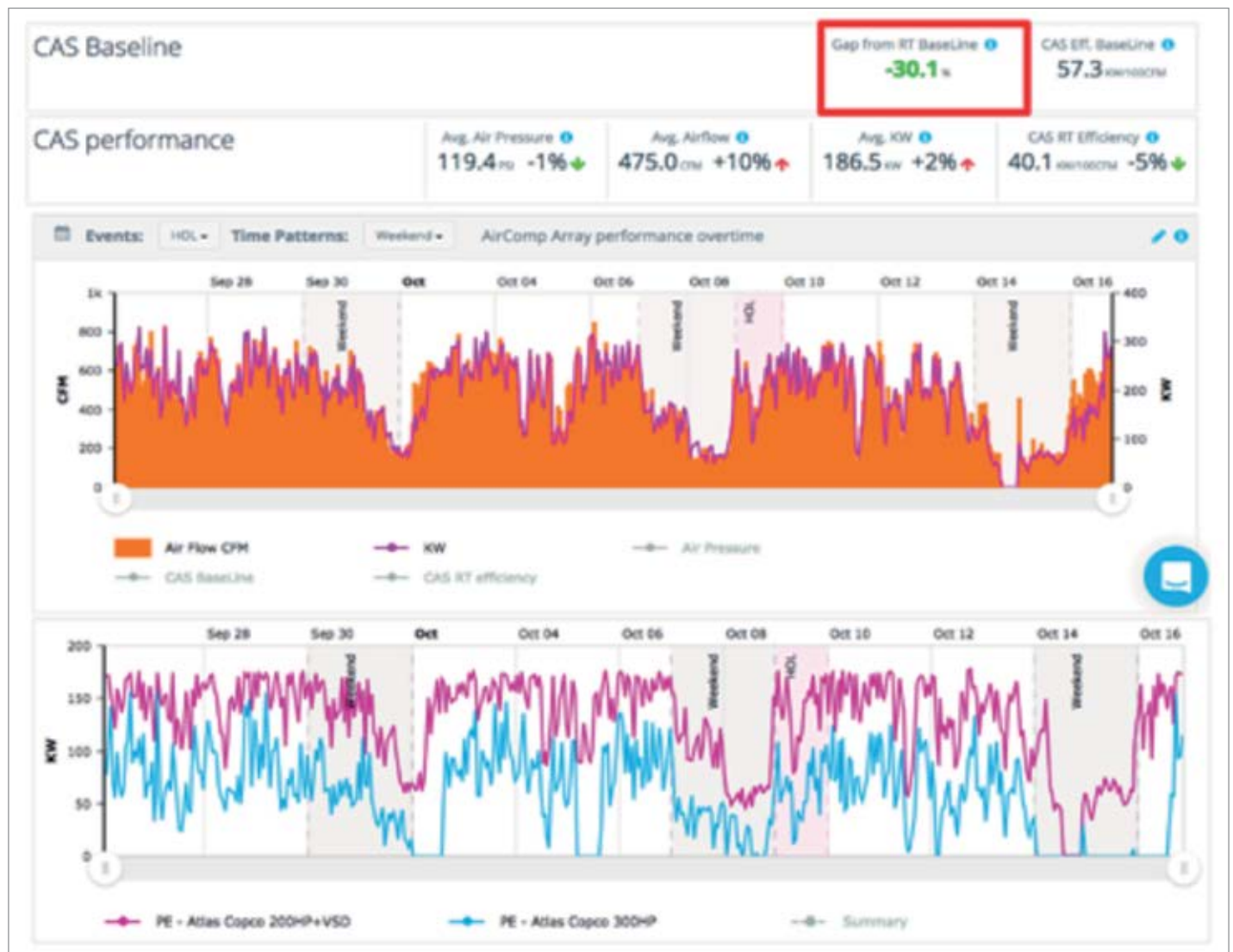
Figure 4: The system specific power has been improved with some simple control system adjustments (Source Lightapp)
