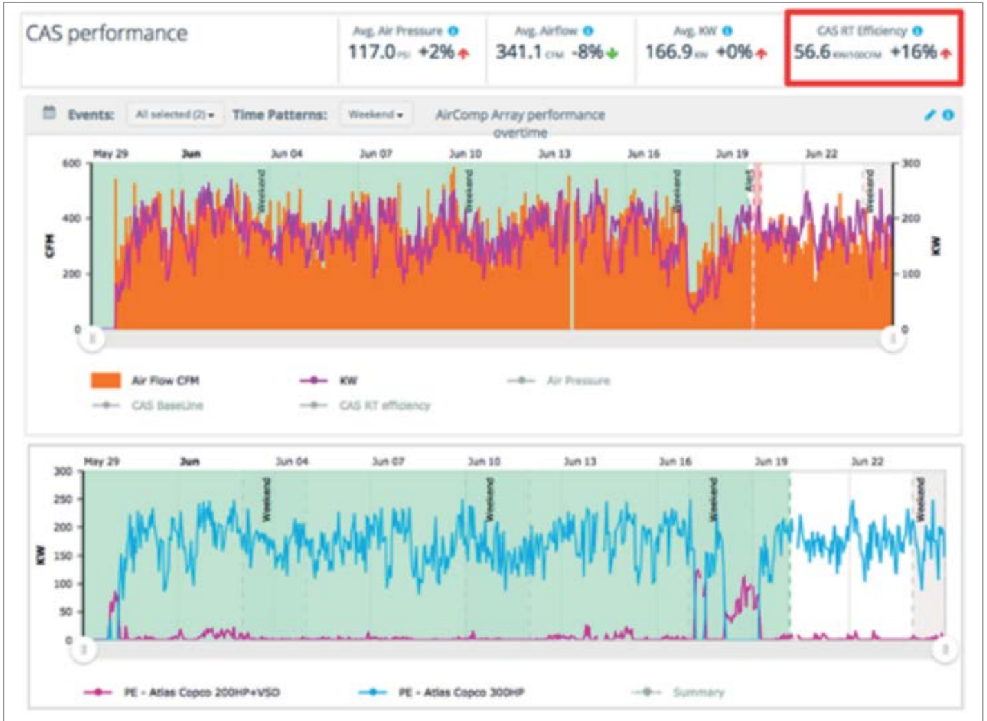
Figure 2: The baseline system efficiency for PepsiCo Fresno, before monitoring, was an unacceptable 57 kW/100 cfm (Source Lightapp)
