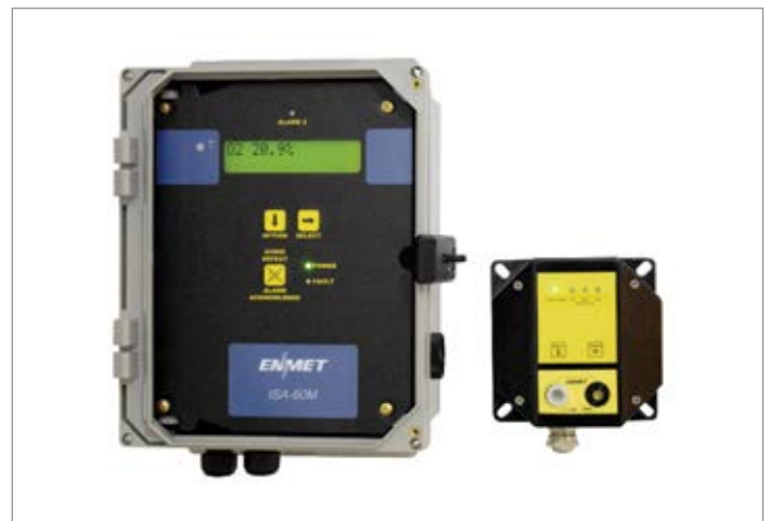
The ISA-60M and MRI-5175 continuously monitors oxygen levels and communicate through a 4-20 mA output.
