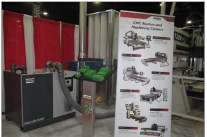
The KOMO booth featured a KOMO 1205 Fusion Twin Table CNC Machining Center supported by an Atlas Copco GHS 900 VSD+ rotary screw vacuum pump.
