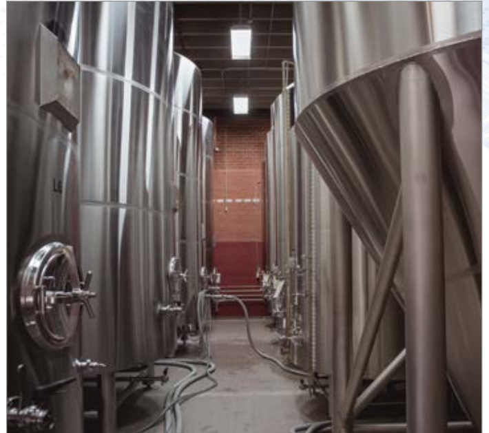
Stainless steel tanks are used to store mash, aerate wort and ferment beer.
