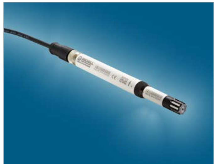
The HygroSmart HS3 sensor uses Michell's polymer tile to give long-term reliable measurements and has an accuracy of 0.8%RH.
