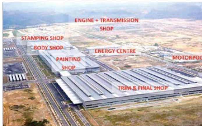
Figure 1: PTMSB Plant Layout
