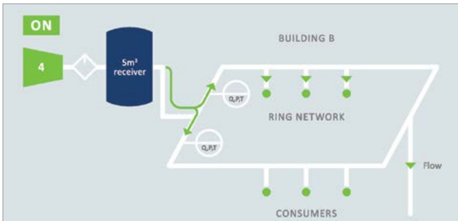
Room B Air Compressor in a "merging traffic" Situation
