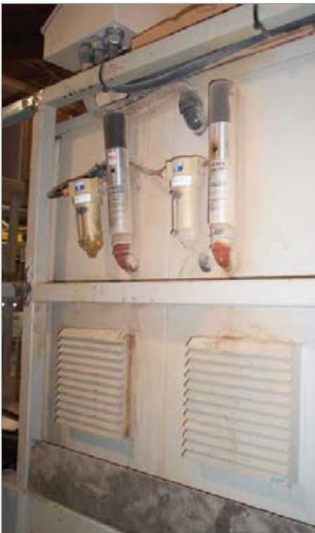
Figure 1: Vortex coolers were discovered during an assessment at a furniture manufacturer.
