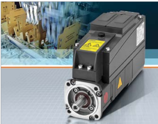
The new Sinamics S120M distributed servo drive system enables decentralized configuration of the drive and integration of the inverter power unit directly onto the driven axis of the motor. Less cabinet space, less cooling energy and shorter cable runs result for the machine builder or production line end-user.
