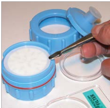
The filter cassette holds three layers of membranes for oil aerosol collection and charcoal tube collect oil vapors. Photo Credit: Trace Analytics, LLC
