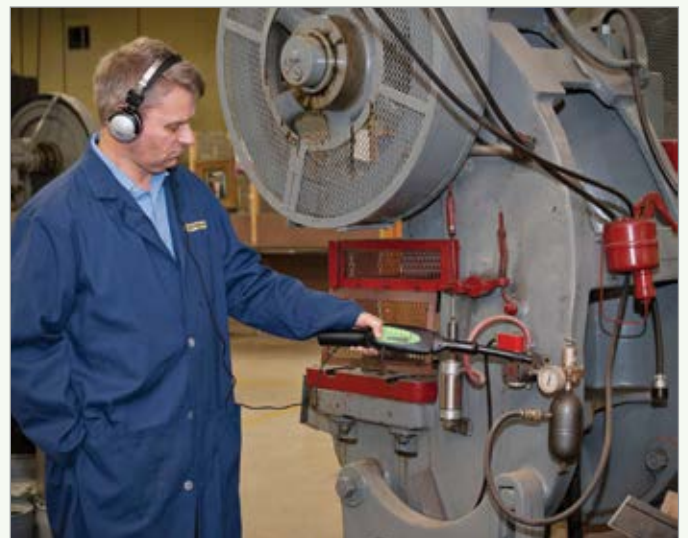
The Spectroline® MDE-2000NC Marksman™ II helps maintenance personnel identify leaks in various industrial applications.
