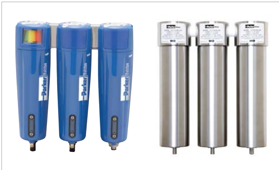
Parker Balston 3-Stage point-of-use filtration modules, in standard and 304 stainless steel housings, will remove contaminants at a very high efficiency - up to 99.99% for 0.01 micron particles and droplets. The final stage of filtration removes all viable organisms with an efficiency rating of 99.9999+% at 0.01 micron (5-log reduction).
