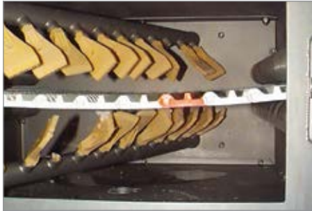
Figure 5: Plastic flat nozzles were used to remove water from conveyors
