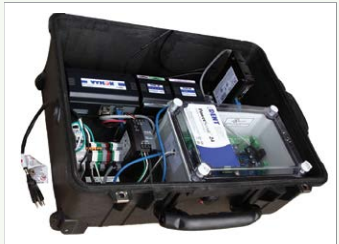
The ReMaster Mobile System for monitoring compressed air systems.
