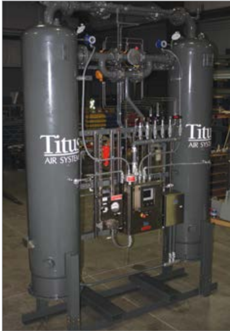
Figure 2: The refinery's Oriad dryer revamped by Titus Air Systems
