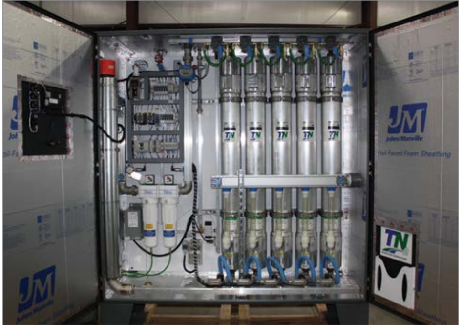
Figure 4: Custom-engineered nitrogen generator that stages from one to five modules
