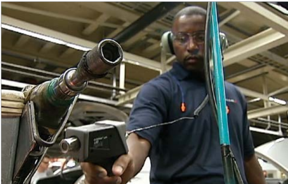
Nissan employs full-time personnel dedicated to identifying and repairing air leaks at each manufacturing facility.
