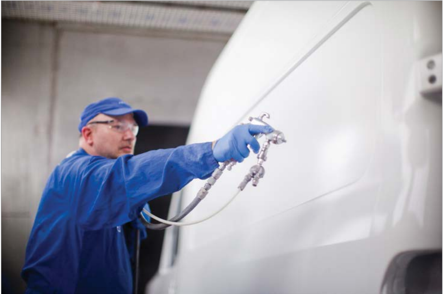
Nissan uses compressed air in a wide variety of applications, including spray finishing.
