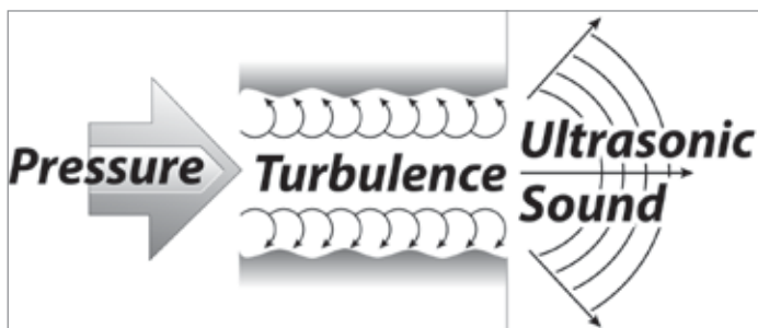
Ultrasonic leak detectors turn inaudible signals into an audible tone.
