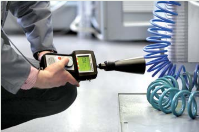
The acoustic horn for airborne probe L 50 for leak detection up to 8 meters.
