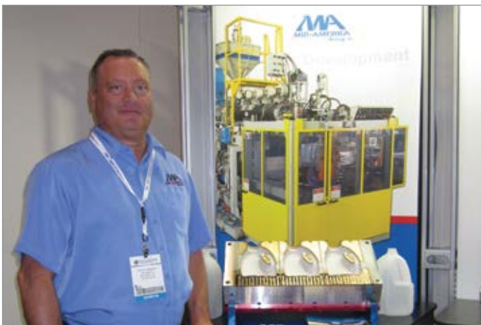
Dave Hubbard from Mid-America Machining standing next to their milk jug mold display. Mid-America designs and manufactures rotary molds, for products like milk jugs typically requiring 100 psig inlet compressed air.
