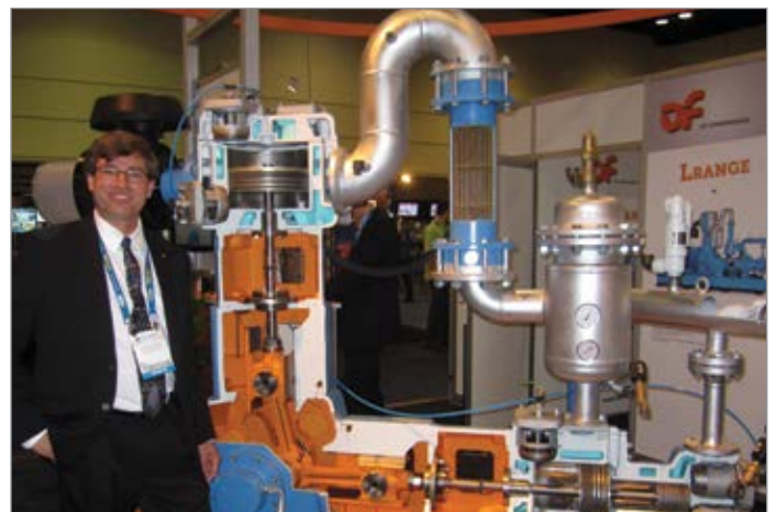
Joe Mashburn, from AF Compressors, next to the CE 24B air compressor able to deliver 353 cfm at 40 bar (590 psi).
