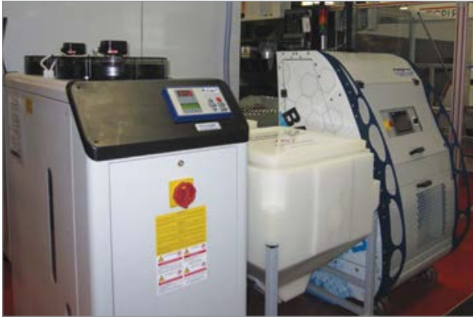
Supporting their injection molding machines, the Negri Bossi booth had a Bauer N 2 IT™ Gas Injection Technology unit alongside a Frigel chiller.
