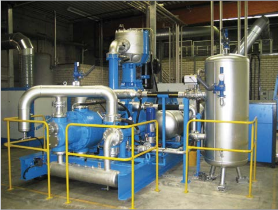
An AF Compressor PET package equipped with the R-Back-5 Air Recycling System
