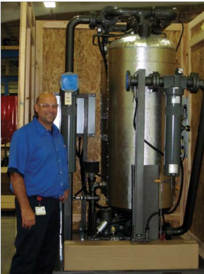
Inspecting the robust packaging protecting an externally heated desiccant dryer before shipment.
