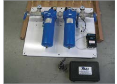
CO monitor panel with oil and odor removal filters
