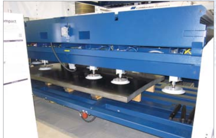
Festo pneumatic cylinders and vacuum venturis allow suction cups to transport metal sheets in the Trumpf LiftMaster.
