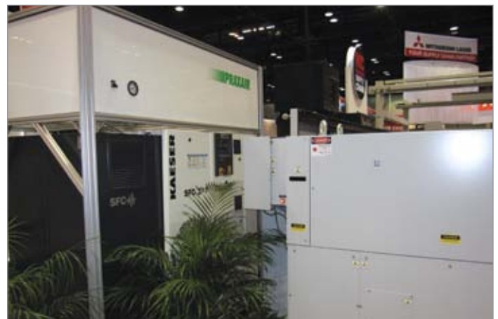
The Mitsubishi Flying Optic CO 2 Laser Assist Gas Supply System with a Kaeser SFC Series rotary screw compressor.
