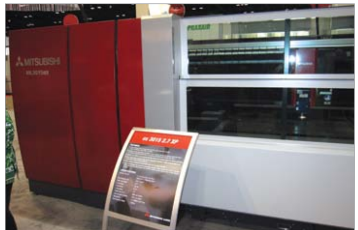
The Mitsubishi High-Speed Flying Optic CO 2 Laser Model ML 3015eX requires nitrogen as the assist gas above 4000 Watts.
