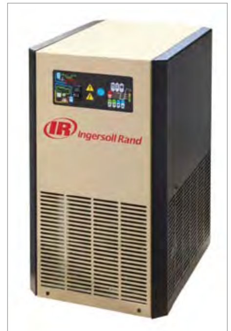
Typically, refrigerated dryers are the most economical to purchase and maintain, and they work well for most general manufacturing applications. These dryers yield air with a pressure dew point between 38 and 50 °F.
