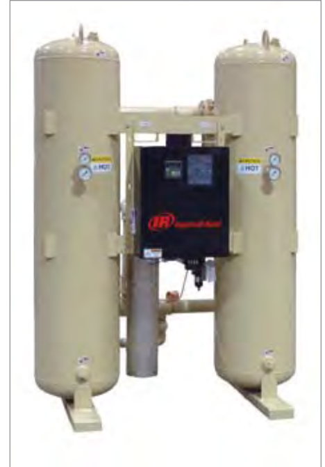
Desiccant dryers, which provide air with a pressure dew point ranging from -40 to -100 °F, use two towers, each filled with desiccant material. While one tower adsorbs the moisture and dries the air, the second tower is regenerated. By alternating tower functions, desiccant dryers provide a constant stream of very dry air.
