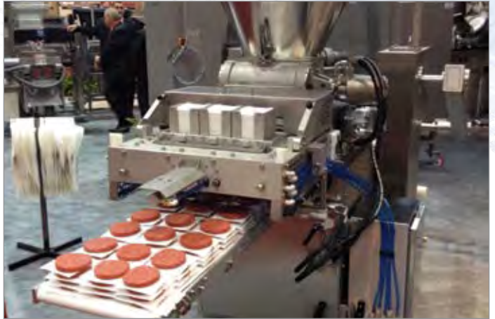
A pneumatically automated machine that creates hamburger patties.
