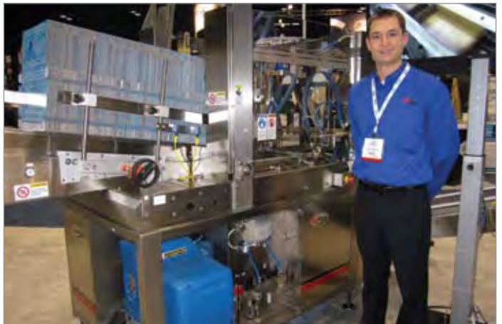
Mitch Kelm, from Delkor, in front of the Trayfecta ® S Series Former rated for 15 scfm at 80 psig.
