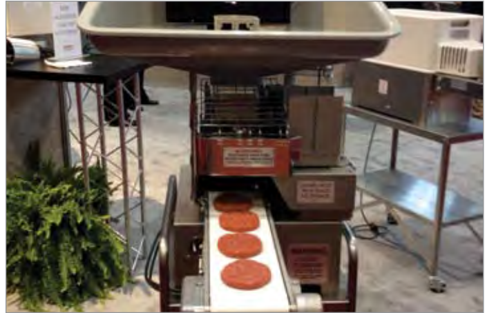
This "Super Patty Machine" uses pneumatics to create 1000 to 2100 hamburger patties per hour.
