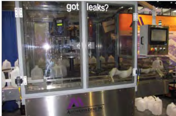
High-speed rotary leak detectors manufactured by Automation Ideas use 25 scfm at 80 psig of compressed air to do up to 240 automated container leak inspections.
