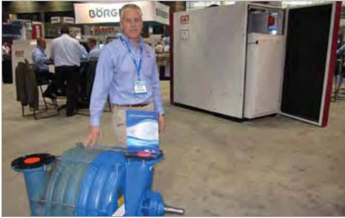
Todd Nelson, from Gardner Denver's Hoffman & Lamson, in front of their remanufactured multi-stage centrifugal blower and the Revolution high-speed centrifugal blower.
