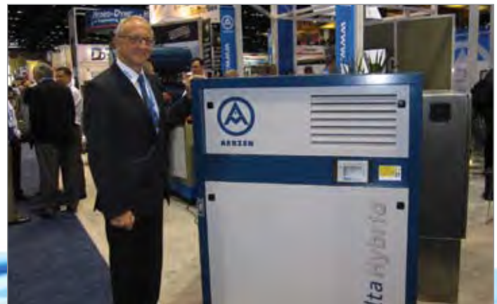
Pierre Noack, from Aerzen, with the Delta Hybrid rotary lobe compressor offering a pressure range from +22 psig to -21 “Hg.
