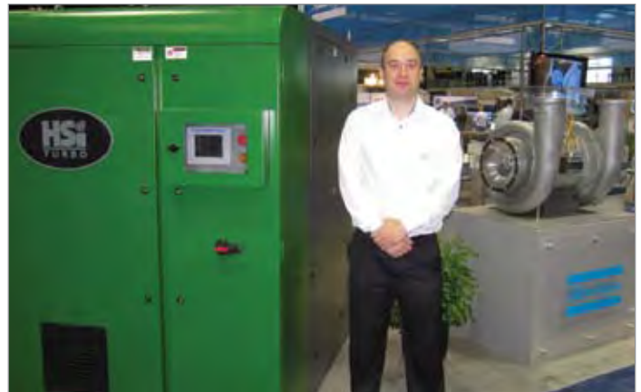
James Elbro and Atlas Copco/HSI Blowers announced the new “Frame 5” 350 hp turbo blower rated for 8000 cfm at 8 psi.
