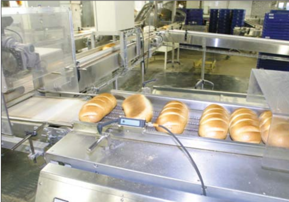
Compressed air is used to blow crumbs off of bread in a commercial bakery.
