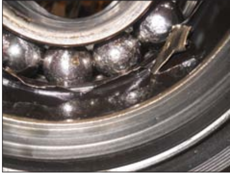
Chemical corrosion evidence on the bearings.
