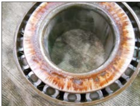
Burnt oil on bearing.
