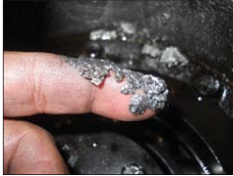
Liquid metal evidence of chemical corrosion.
