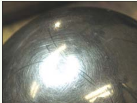
Scratches on bearing.
