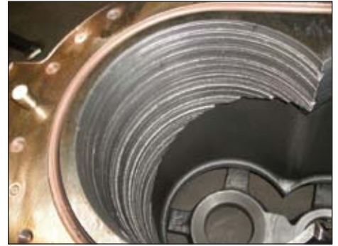
Damaged rotor housing.
