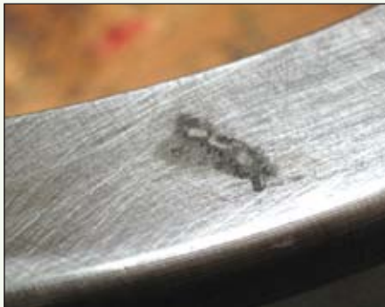
Damage mistaken as electrical arcing.
