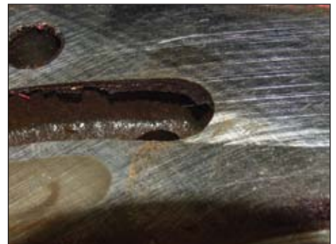
Burnt oil residue in oil port.
