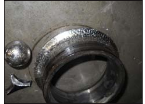
Corrosion on the bearing and bearing race.
