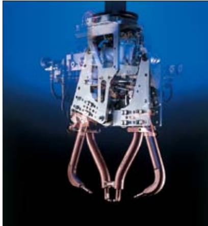
Fig. B: Servo-pneumatic drive system by Festo for welding tongs
