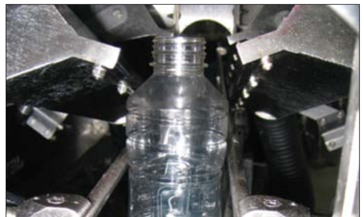
Water Container Drying: A facility filling 5-gallon water containers replaced compressed air with a direct-drive centrifugal blower. Photo provided courtesy of JetAir™ Technologies.
