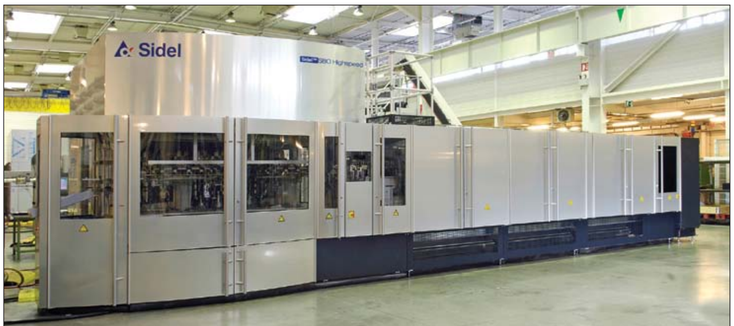
Pressure drops in the pneumatic circuits of blow molding machines can be as high as 50 to 75 psig. Some manufacturers, like Sidel, design circuits to effectively manage this issue.
