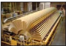
View of the particleboard cooler
