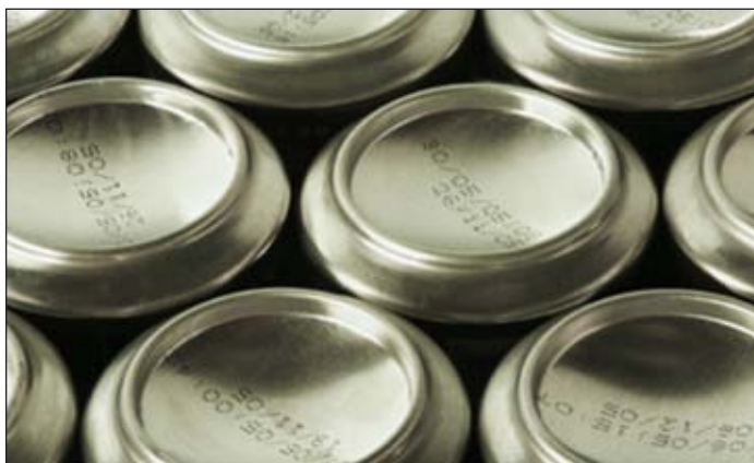
Can Printing: Printing on wet cans results in illegible lot/date codes and "can bursts" ruining packaging and unsellable pallets of product. Centrifugal blowers and air knives replace compressed and improve drying performance. Photo provided courtesy of JetAir™ Technologies.
