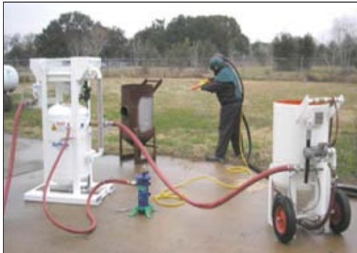
Figure 1. Typical large “Sand Pot” most often used for larger material treatment, particularly outside.
