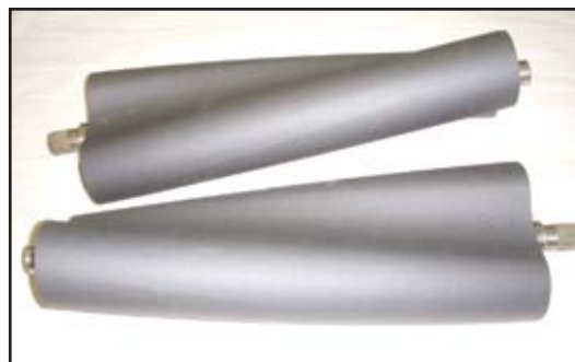
Unusual twisted rotor design in Hampton supercharger combines some of the characteristics of older Roots-type blower and screw type.
