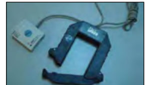
Hobo data logger and current transformer.
