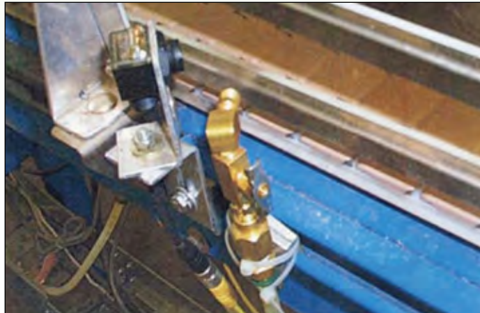
Figure 1 — Note the blow is still on while there is nothing on the line.
