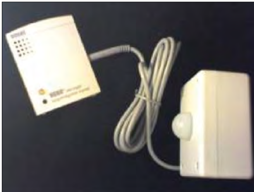
#9 An occupancy sensor can help determine the amount of time lights are on without people in the area.
