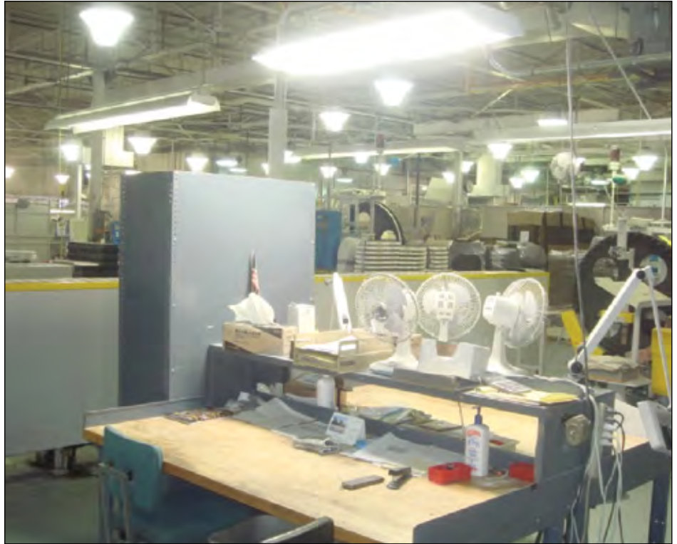
#5 Lights on without workers and excessive lighting in non-work areas.
