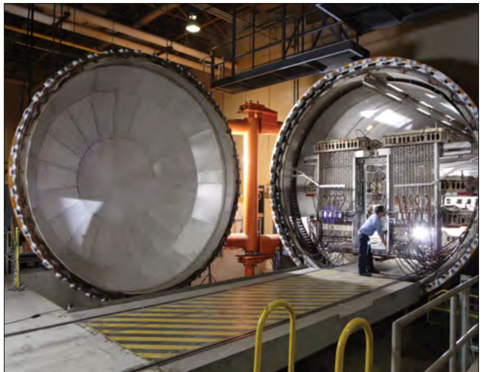
This massive autoclave requires 69,000 cubic feet of nitrogen at a flow rate of 3,450 cfm to fill to 100 psi in 20 minutes.
