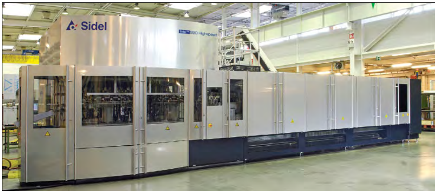
The Sidel SBO 34 Highspeed blows 61,200 small bottles per hour (from 0.2 to 0.7 L).
