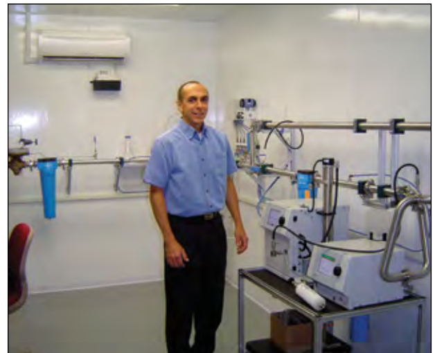
Mark Honath, Senior Engineer, Research & Development, SPX Dehydration & Filtration, demonstrates the SMPS (Scanning Mobility Particle Sizer) System within the ISO 12500 Part 3 Test Lab.
