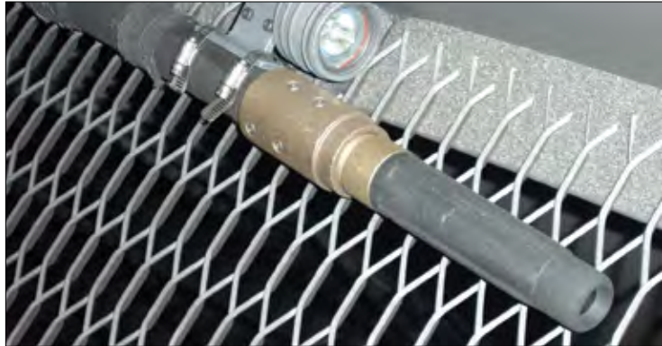
Blast nozzle erosion of even 1/16th of an inch can increase the air consumption by 30%. A 10 psi plant pressure increase will increase the air consumption by 9%.
