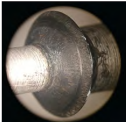
Figure 6: Over-molded poppet removed from kneeling module after 2 million cycles
