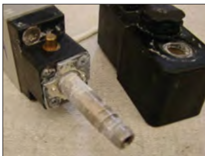
Figure 8: Salt Spray Testing performed on pilot operator and coil
