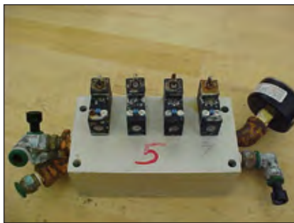
Figure 7: Kneeling module after Salt Spray Testing
