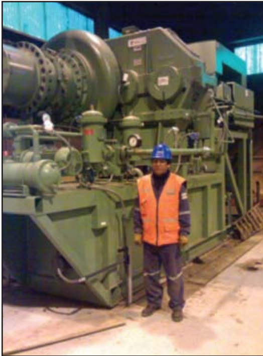
The new centrifugal oil-free compressor with extended turn-down capabilities
