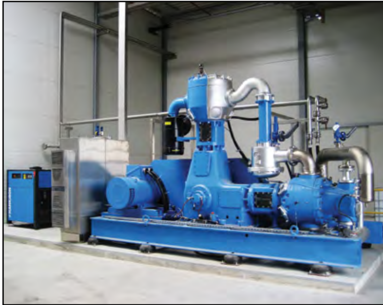
The AF three-stage oil-free reciprocating compressor design
