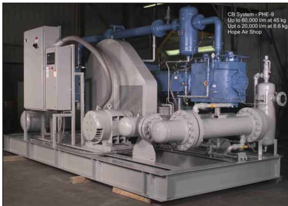
200 HP Booster Package for Milk Bottle Producer
