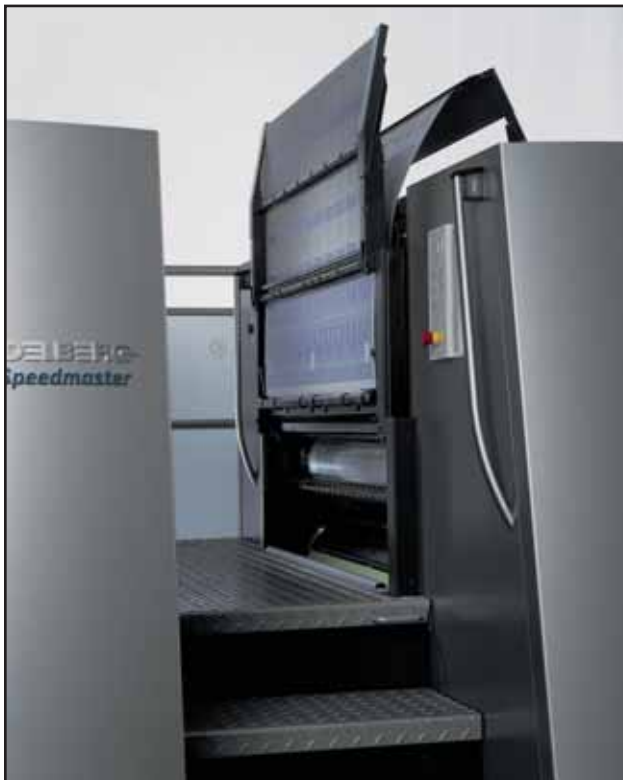
The auto advance feature for printing plates uses pneumatics (Illustration: Heidelberger Druckmaschinen AG).
