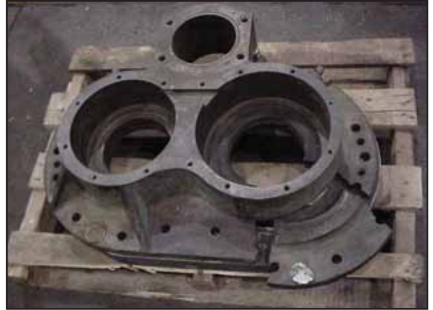
Cracked air end housing plate.
