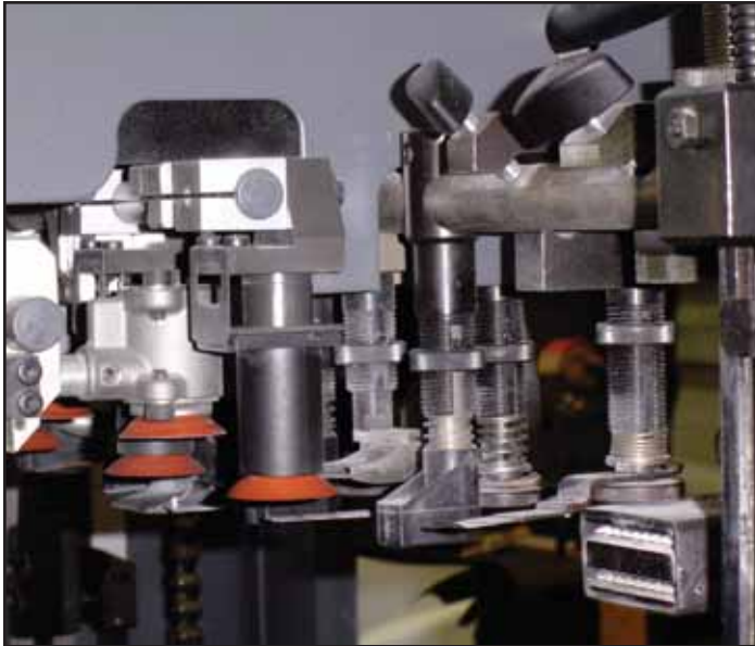
The suction head of the sheet feeder with both lifting suckers and a horizontal blow port.
