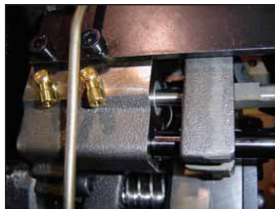
Pneumatic piston controls the position of the blanket cylinder.
