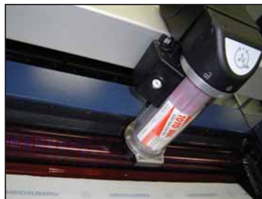
The ink dispensing unit uses pneumatics.
