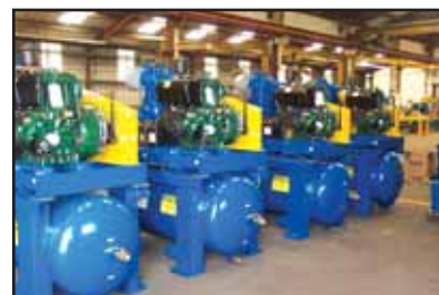
McKenzie Diesel-Driven Cold-Start and Black-Start Air Compressors
