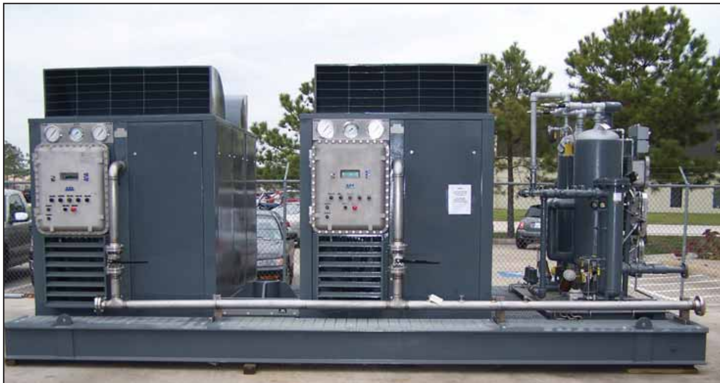
Offshore rig package of two 200 horsepower air compressors and an internally heated desiccant air dryer. Built with explosion-proof panels, offshore paint, and all seal-welded construction. Installed on an offshore rig, west of India.
