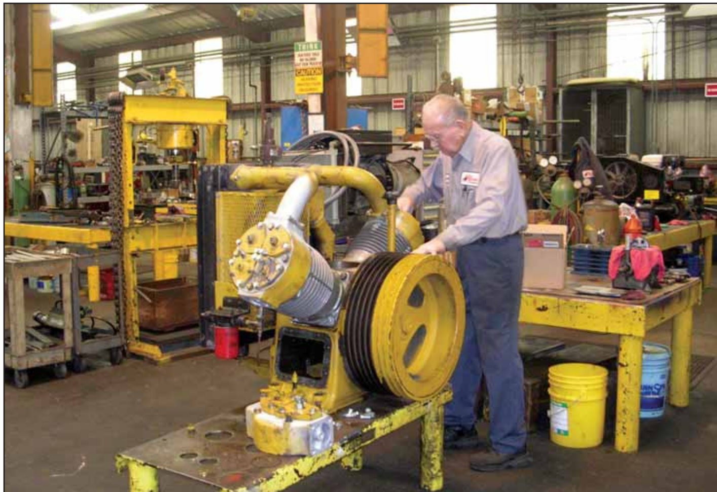
Re-building a high-pressure LeRoi compressor
