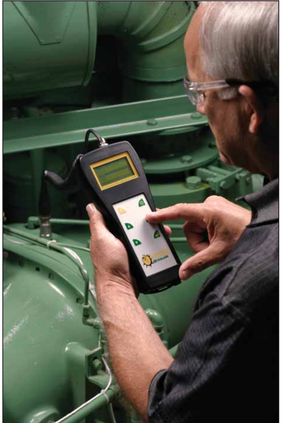
This hand-held condition monitor trendlines the performance of key compressor components over time to provide advanced indication of equipment failure.
