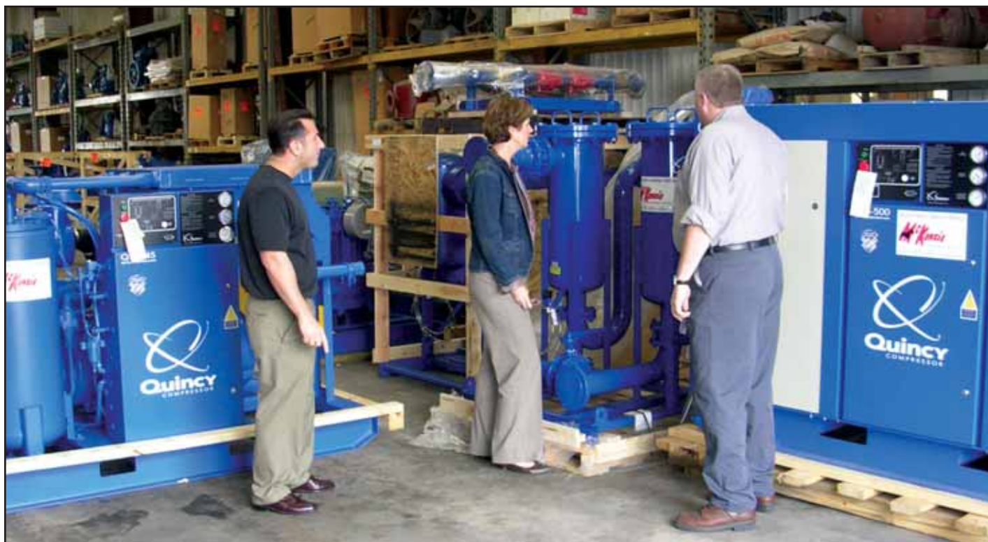
Inspecting Quincy OSI Rotary Screw Compressors and Air Treatment Skid Before Shipment
