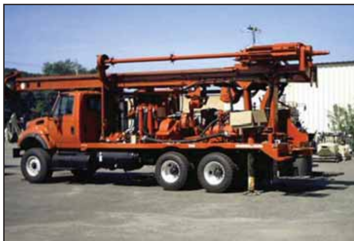
Mobil drill rig with two Ingersoll Rand 750 cfm @ 350 psi air compressors
