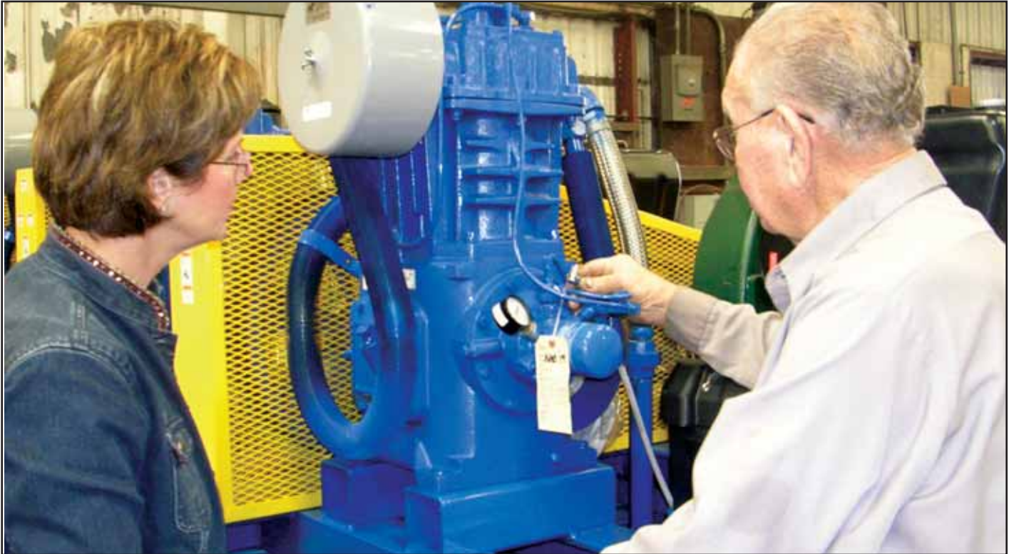
Mary Ann Goode and Raymond Roberts inspect a Quincy QR-25 Reciprocating Air Compressor
