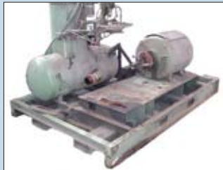
Step 2: Air compressor is stripped for bench rebuilding of major components.
