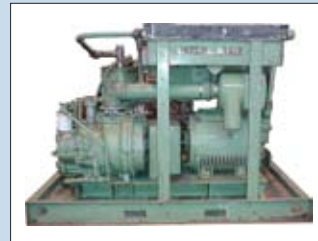
Step 4: Air compressor is fully tested and ready for paint.
