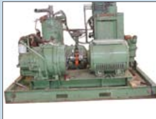
Step 3: Air compressor is assembled from rebuilt components.
