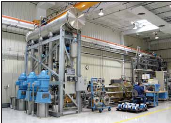
ISO 17025 certified calibration rig allows Endress+Hauser to deliver highly reliable measuring instruments with fast delivery times to our customers throughout North and South America. The large calibration rig above handles flow tubes up to 12 inches in diameter.
