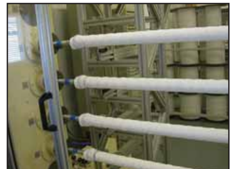
BEKO membrane bundles in production in Bend, OR
